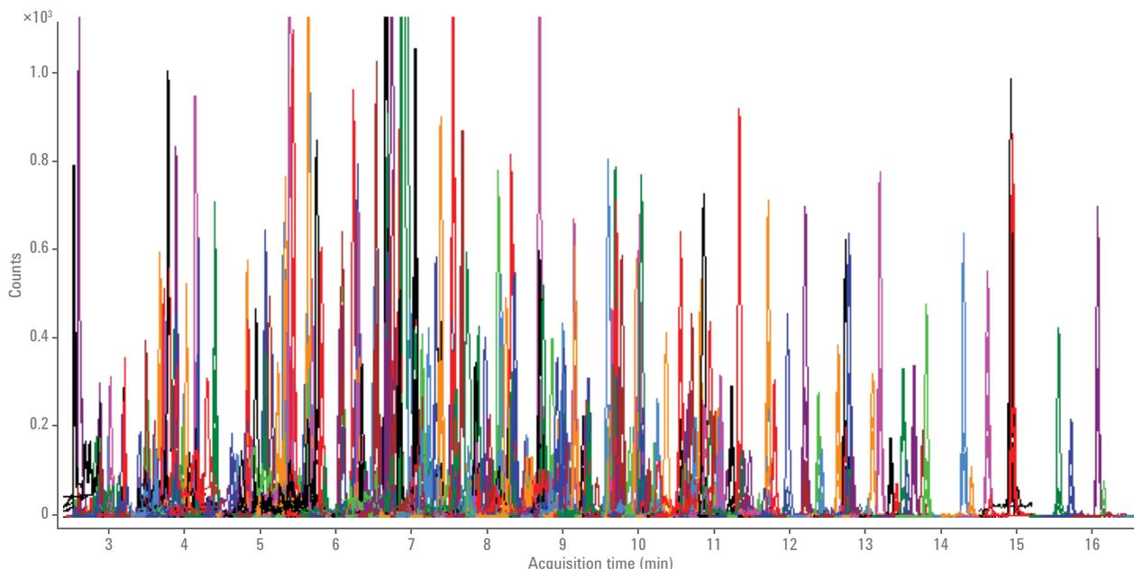
**Figure 2.** The signal response of the Agilent Ultivo Triple Quadrupole LC/MS for 246 pesticides spiked in black tea matrix at 5 ng/g (1 ppb).
